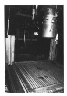
The mill featured a sophisticated method of grinding the fruit and a press capable of applying pressure at three speeds. This model, using all steel construction, was considered the finest screw cider press ever made. In the twentieth century, the hydraulic press came into widespread use. Thus, B.F. Clyde's Cider Mill is representative of the final and finest mills using the mechanical screw press.
